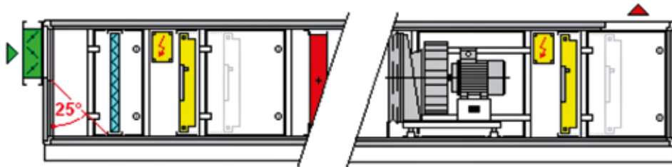
Diagram of the electrostatic filter with removal from the front, placed upstream and downstream of the fan.
